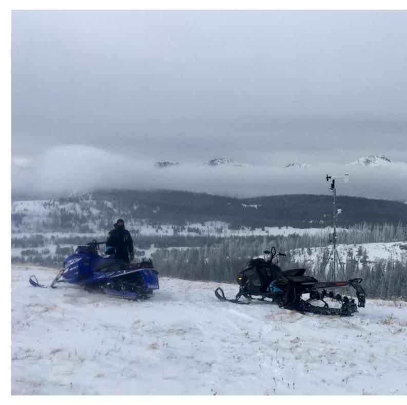
We put up the Taylor Fork Weather station today. It measures wind direction and speed, RH, and temperature. Coupled with the <u>Carrot Basin SNOTEL</u>, this gives us a good idea on what is occurring in this range. Photo GNFAC
