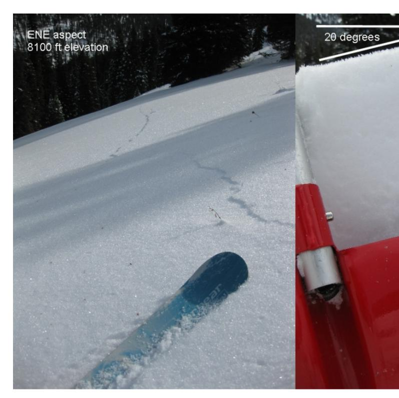
This slope collapsed and cracked when skiers approached it. If the slope had been steeper than 30 degrees it would have avalanched. These are clear signs of unstable conditions. Photo: K. Birkeland
