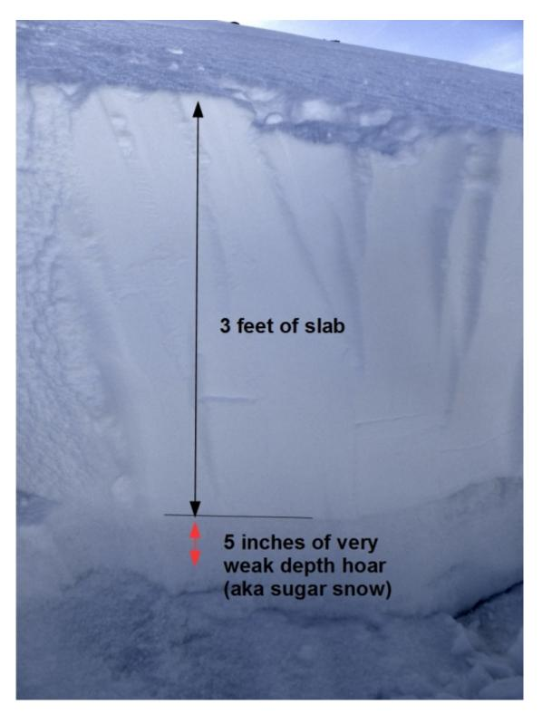
This slope had very thin snow considering the nearby Fisher Creek SNOTEL has over 10 feet of settled snow. This thin snowpack led to the formation of very weak <u>depth hoar</u> (6-10mm in size and Fist+ hardness). Photo: GNFAC
