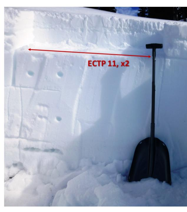
This pit was dug on a SW facing slope. It broke on a layer of facets and surface hoar about a foot deep (ECTP 11 and 12). This layer is not widespread, but is worth looking for since avalanches are possible on it. Photo: GNFAC
